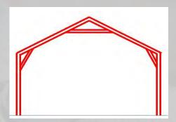
The Structural steel building frame consists of columns and rafters. The column and rafter are typically tapered being narrow at the foundation and peak and wider at the rafter/column connection.
